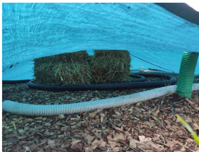
Figure 3: nylon cover, aeration and recirculation pipes detail
